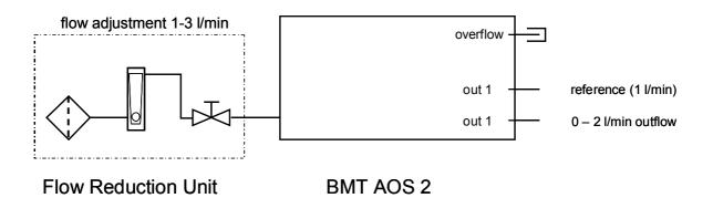
The Flow Reduction Unit consits of a particle filter, a flow meter and a throttle valve. The throttle valve can be used to adjust the total flow through the AOS 2. Please note: The outflow on OUT 2 depends on the flow rate of the reference monitor on OUT 1. In case on a reference monitor BMT 932, the flow on OUT 1 is 1 l/min.
