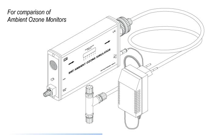
The BMT AMBIENT OZONE SIMULATOR AOS 1 is a simple means to comparing two ambient ozone monitors with each other.
