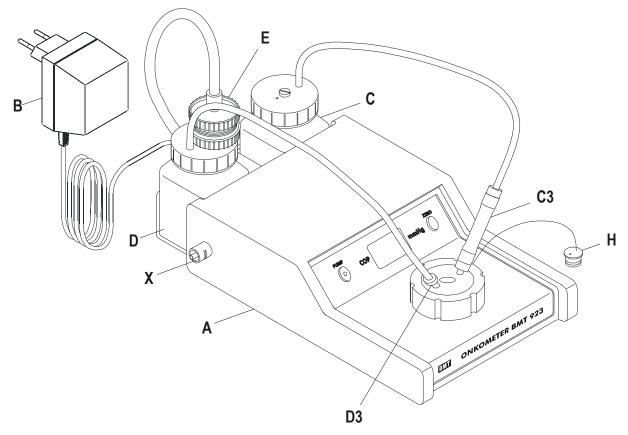
The caps of the plastic bottles are different: The right cap (see sketch) is that of the rinse bottle ( $\mathbf{C}$ ) containing fresh saline. The other cap is that of the waste bottle ( $\mathbf{D}$ ) into which the waste from the sample chamber is sucked with the help of the internal electric vacuum pump when the push button PUMP is pressed. This cap has a Luer bore in which the air filter ( $\mathbf{E}$ ) is plugged in.
