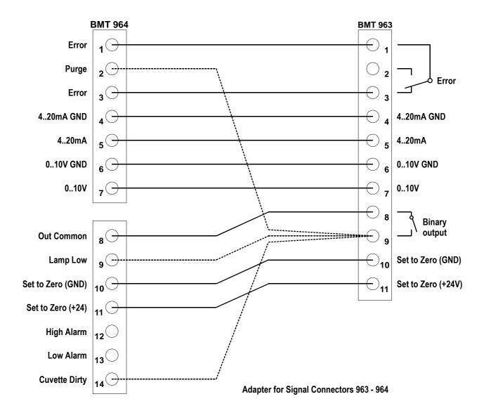
This adapter helps to replace an OZONE ANALYZER BMT 963 with an OZONE ANALYZER BMT 964. The binary output of the BMT 963 (pin 9) depends on what has been ordered. The function is marked on top of the cover. For detailed description of the signals please refer to the manuals.
