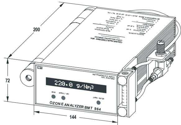
The OZONE ANALYZER BMT 964 BT is a portable instrument in an enclosure according to DIN 43 700.
