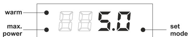
Three LEDs on the digital display additionally are signaling the status as shown above.
