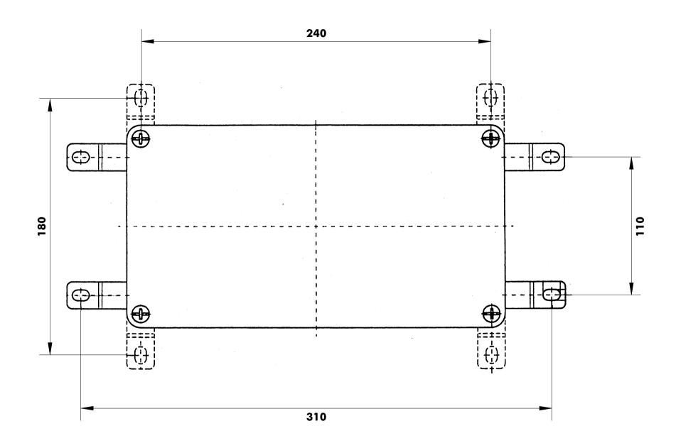
OZONE-IN-WATER SENSOR BMT 963 / 964 AQ Mounting Holes
